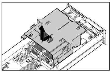
Figure 1-15: Removing the processor baffle
